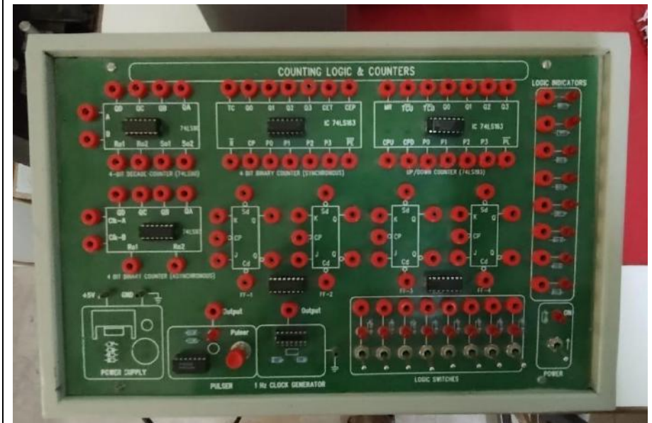
4-bit binary Up/Down counter by using 74193 IC
